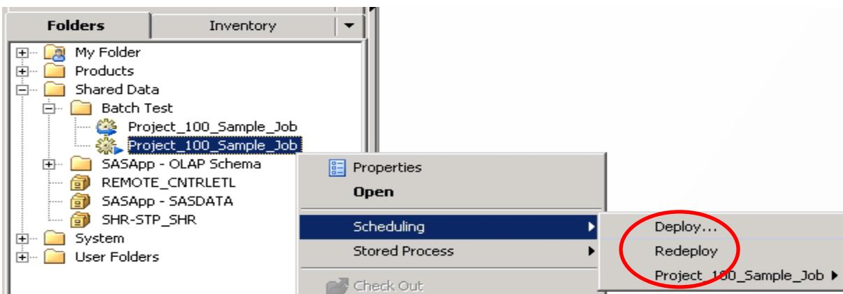
**Figure 5. Manually Redeploying a Job**
